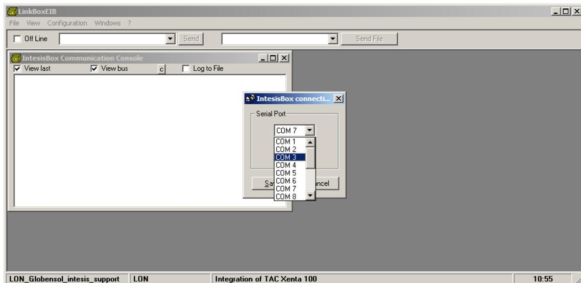
3. Click the checkbox next to *Offline* word below LinkBox Menu. It should change to *Online*, and some output must appear at *IntesisBox Communication Console* window.
