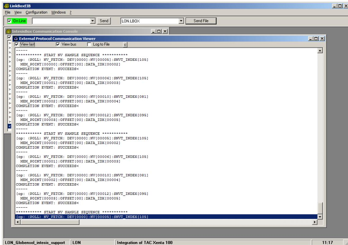
These pose as the query commands the IntesisBox is triggering to the LonWorks device being integrated.
