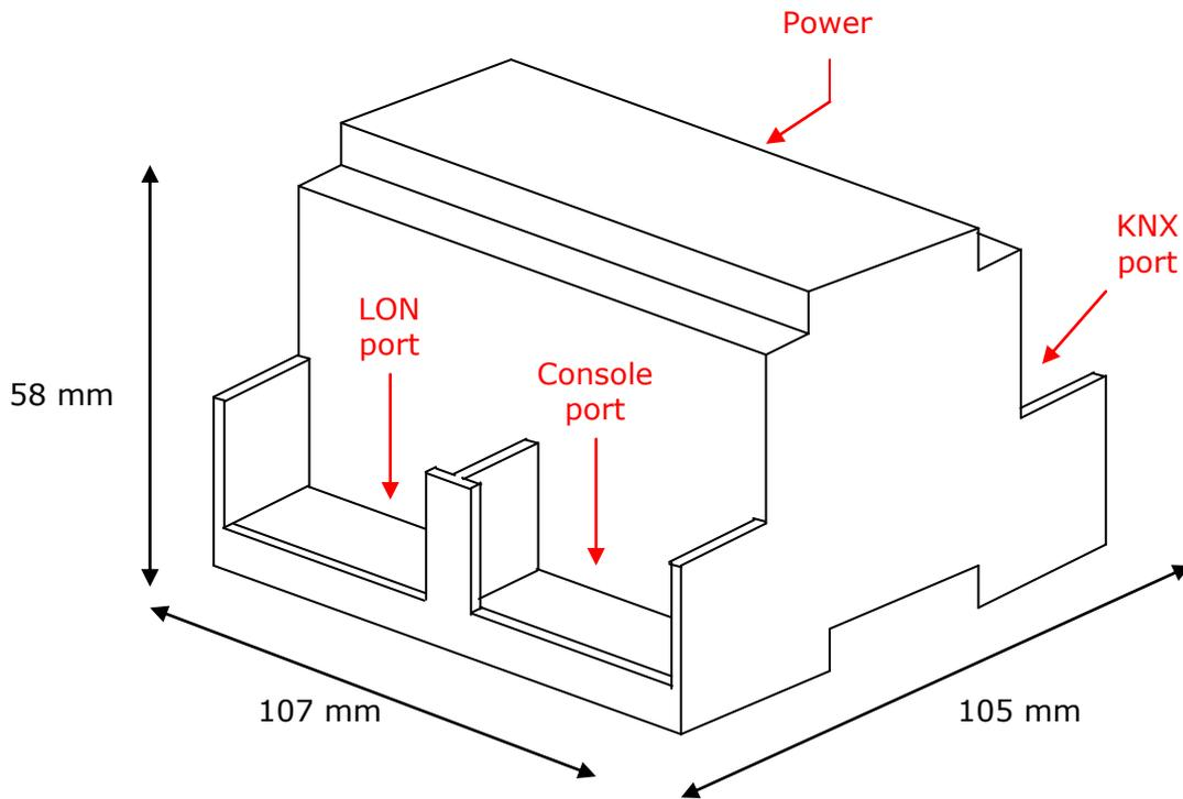
Recommended available space for its installation into a cabinet (wall or DIN rail mounting), with space enough for external connections:
