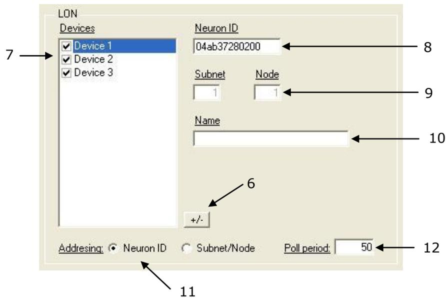
6. Use this button to define the number of LON devices to integrate. Remember the limitations: just 64 devices in IntesisBox basic model, and 128 devices in IntesisBox extended model.
